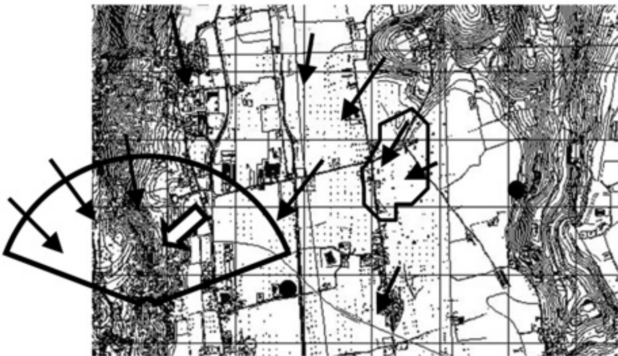
Figure 4 : Topographic map indicating the location of P9p (dot on the left) and K13p (dot on the right) sites. Black arrows indicate the subterranean flow direction. The R.R.Z. (Restricted Respect Zone) and the recharge area of the karstic site are reported too. The thick white arrow indicates the Pantena stream (scale 1:10000).
